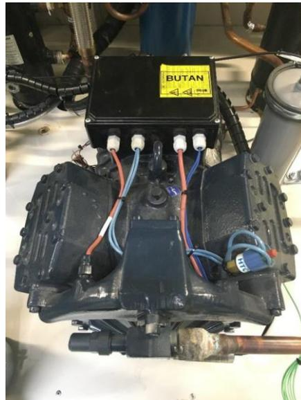
Figure 9. The prototype DORIN compressor used by Bamigbetan et al. [11].
