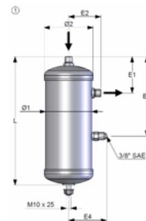
Figure 27: Diagram of CARLY oil separators and table with dimensions.
