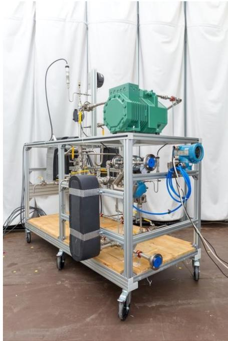
Figure 4. HTHP with BITZER compressor proposed by Fleckel et al. [9].
