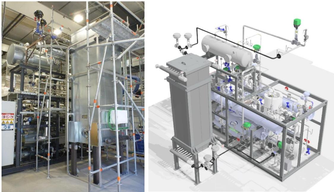
Figure 13: LH-TES connected to the steam generator in the laboratory at DLR site. Test setup during installation (left) and 3D-drawing showing the system layout and pipe connections (right)
